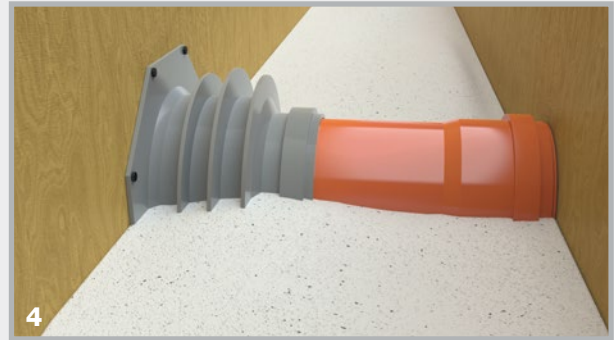
4 Concreting and careful sealing
