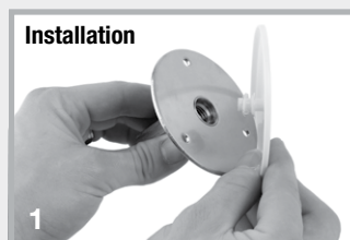
1 Remove protective cap of fixed earthing terminal
