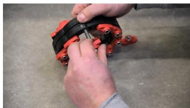
Insert the screw through the holes in both rubber ends to fix the closed chain.
