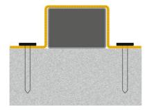
Place the swelling tape grid carefully over the swelling tape without damaging the protective sheating.
