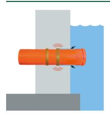
Pull off silicone paper and affix 2 rings of **MASTERSTOP SK** around the pipe to be waterproofed.
