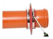
Apply lubricant to the clamping range of the strap, then tighten the clamping straps sufficiently using a screwdriver to prevent the RONDO Protect sealing collar from shifting.
