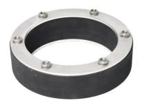
Supply takes place completely ready to be installed. The **MASTER-RING** gasket insert consists of two pressure plates, a rubber part and the appropriate screws and nuts. The pressure plates, the screws and the nuts are made of V2A stainless steel.
