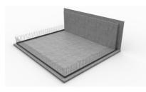
The cavity wall elements are positioned with VB joint sheet metal acting as the foundation/wall waterproofing element until reaching the corner area.
