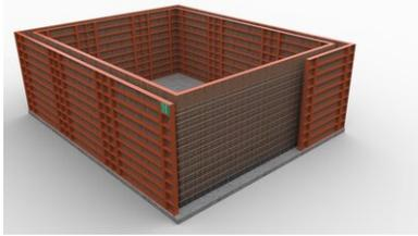
The in-situ concrete element is positioned with VB joint sheet metal acting as the foundation/wall waterproofing element.
