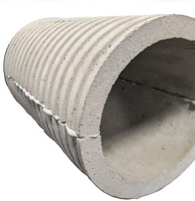
Place the top shell and press on it so that the adhesive squeezes out of the joint.
