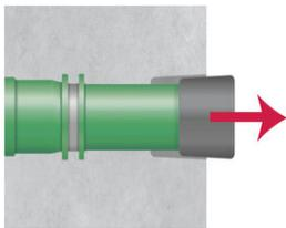
The socket ring is removed before the next pipe is connected.
