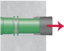
The socket ring is removed before the next pipe is connected.
