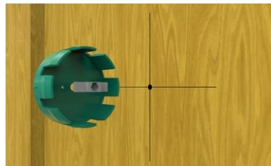
Insert the **FIX screw adapter** into the **FIX formwork aid** and press it in firmly.
