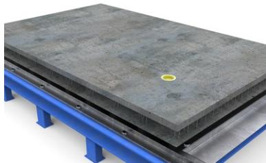
After that, the reinforcement can be laid and the two shells concreted.
