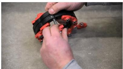
Insert the screw through the holes in both rubber ends to fix the closed chain.
