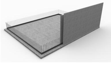
The first cavity wall element is positioned with VB joint sheet metal acting as the foundation/wall waterproofing element.
