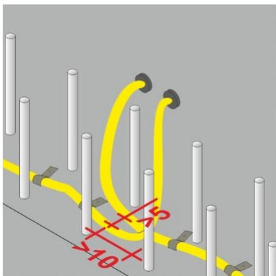
Fastening packers are screwed into the ends of the injection hose sections up to the thread end and fixed to the formwork surface. The position of the fastening packer should ensure permanent accessibility (floor structure and Technical Building Equipment must be taken into consideration). The fastening packers have closure plugs in 2 different colours. These are used for marking of the pairs used for the individual hose sections.
