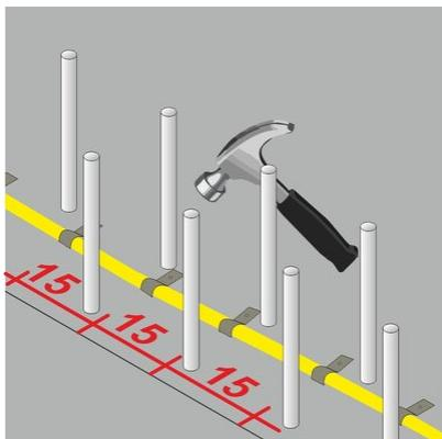
**MASTERTUBE "YELLOW"** must be fixed in such a way that it cannot shift neither before nor during concreting. It can be fastened by using metal clips or plastic fastening clips. The distance between either type of clips must not be more than 15cm in longitudinal direction. On very uneven surfaces and at each change of direction, the distance should be halved.
