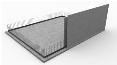
The first cavity wall element is positioned with VB joint sheet metal acting as the foundation/wall waterproofing element.
