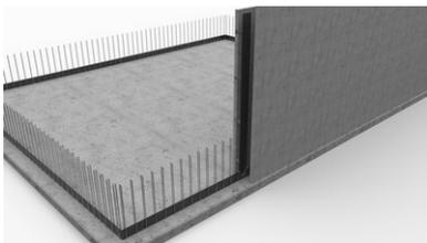
Installation of the **SFG profile** is complete; the next cavity wall element can be placed.
