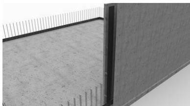
The **SFG profile** is set vertically and overlapped with the joint sheet metal (overlap  $\geq 5$  cm).
