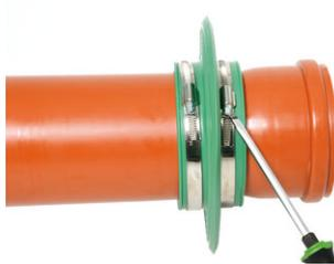
Apply lubricant to the clamping range of the strap, then tighten the clamping straps sufficiently using a screwdriver to prevent the **RONDO sealing collar** from shifting.
