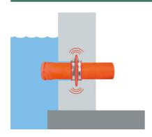
Der RONDO Protect Sealing collar is positioned in the center of the concrete component.
