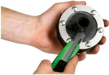
Simply cut off the pushed-through ring using a cutter
