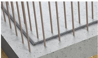
In the corners, the swelling tape grid must be released in order to ensure a continuous firm fixation on the substrate. In the case of butt joints in the straight line and the use of swelling tape grids, the joints of swelling tape and swelling tape grid should always be made in a staggered position.
