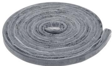
Since the **MASTERSTOP "LONG TIME"** is supplied with a protective sheathing, the swelling tape can only be fastened by using a special swelling tape grid. The substrate must be clean, dry and free of loose parts. Apply the **MASTERSTOP "LONG TIME"** in the middle of the joint to the concrete surface and fix it. The later concrete cover must be at least 8cm. The swelling tape must be bordered by reinforcement on both sides. Minimum distance to the reinforcement: 5cm.
