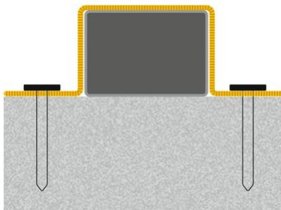
Place the swelling tape grid carefully over the swelling tape without damaging the protective sheathing.
