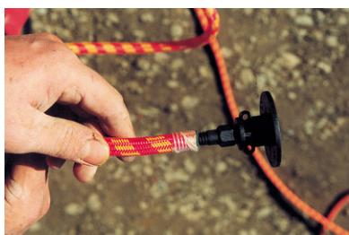
After the hose has been cut to length, screw the respective connecting pieces fully into the hose (as far as they will go) - the image shows our fastening packers.
