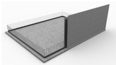
The **SRF profile** is set vertically and overlapped with the joint sheet metal (overlap  $\geq 5 \text{ cm}$ ).
