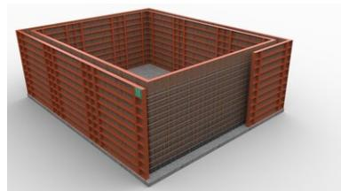
The in-situ concrete element is positioned with VB joint sheet metal acting as the foundation/wall waterproofing element.
