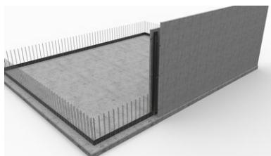
Installation of the **SRF profile** is complete; the next cavity wall element can be placed.
