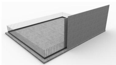
The cavity wall element is positioned with VB joint sheet metal acting as the foundation/wall waterproofing element.
