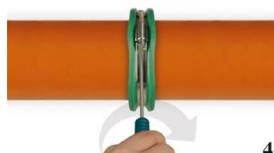
The clamping strap is tightened to approx. 5-6 Nm torque to prevent the **RONDO Base** from shifting during concreting.
