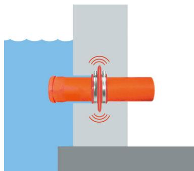
Der **RONDO Protect Sealing collar** is positioned in the center of the concrete component. It reliably and permanently prevents water penetration at the outer pipe wall.
