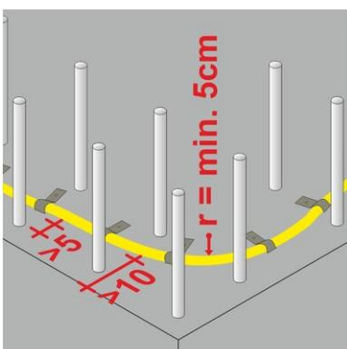
Changes of direction must be carried out with a sufficient bending radius in order to avoid damage to the hose or an obstruction of the overall injection.
